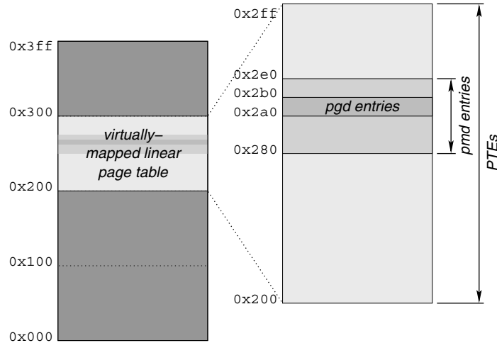
Figure 4.20. Effect of self-mapping entry on virtual address space.
