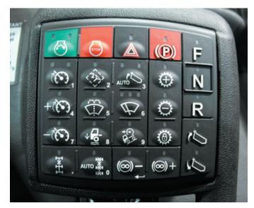
FIGURE 7-23 A keypad used to start a machine.
