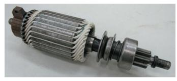
**FIGURE 7–11** A typical armature and how the loops of wire are embedded into the core.
