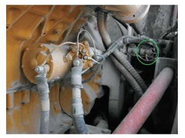
FIGURE 7-27 A heavy-duty starter relay.
