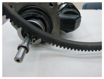
**FIGURE 7–3** A starter assembly engaging with a flywheel ring gear.
