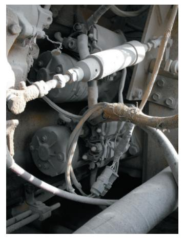
FIGURE 7–4 A double starter assembly arrangement.
