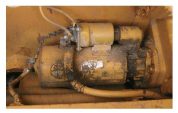
**FIGURE 7–2** A typical arrangement of a heavy-duty electric starter on a diesel engine.
