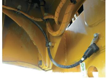
FIGURE 7-21 A properly secured battery cable.
