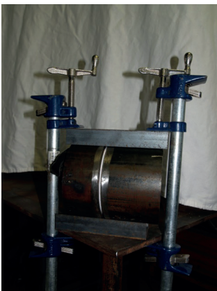
FIGURE 7-5 Channel Iron Used for alignment.
