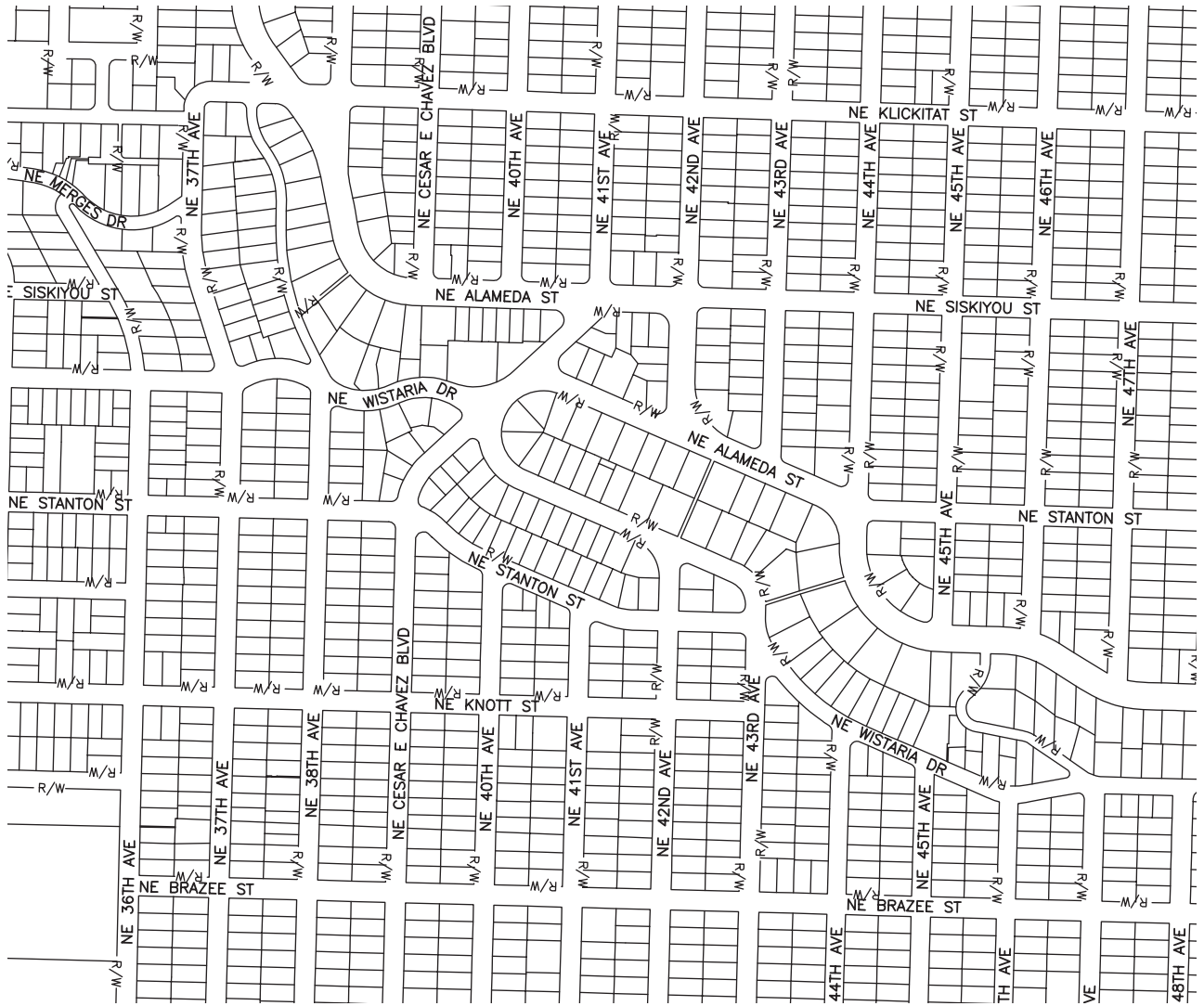
Figure 1-11. A portion of a Portland, Oregon cadastral map. (Courtesy of the City of Portland, Oregon)
