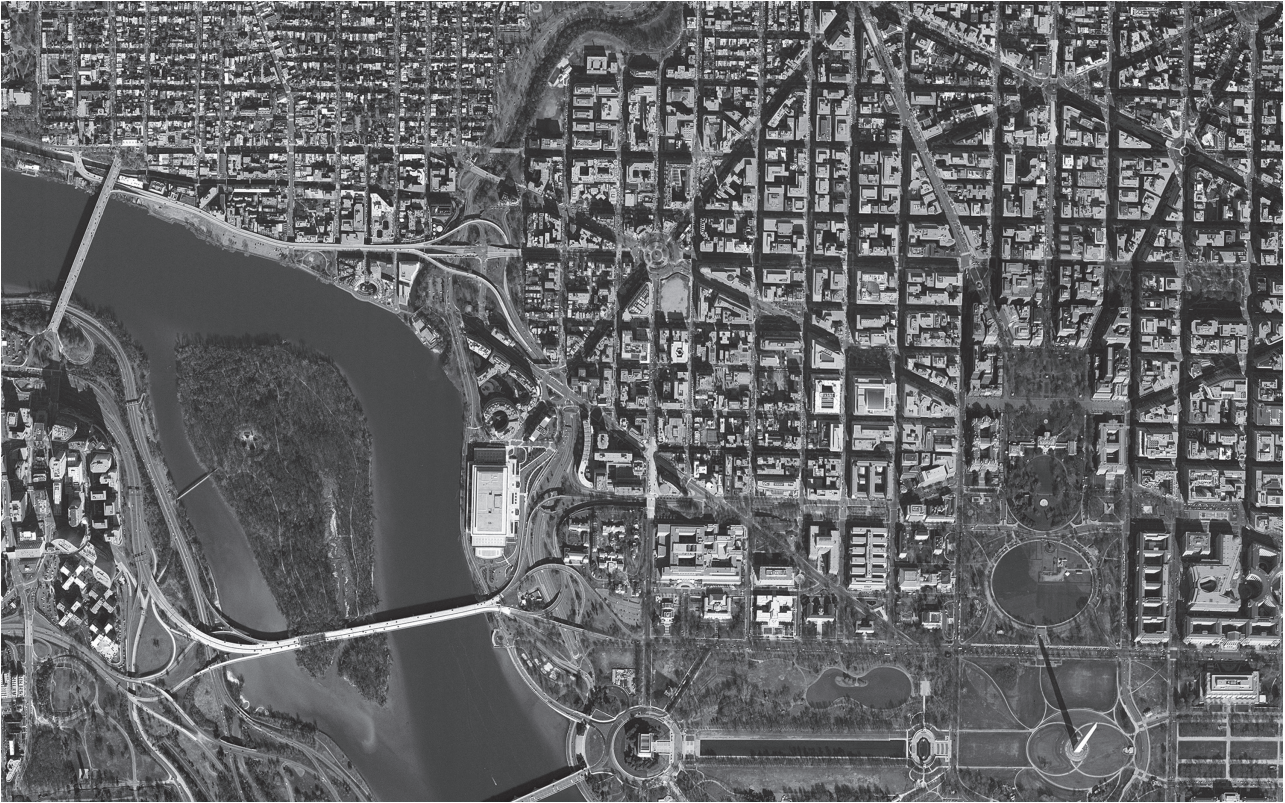
Figure 1-6. This aerial photograph of the District of Columbia can be used to create a photogrammetric map.
