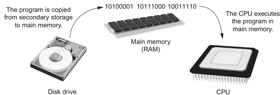
When a CPU executes the instructions in a program, it is engaged in a process that is known as the *fetch-decode-execute cycle*. This cycle, which consists of three steps, is repeated for each instruction in the program. The steps are:
