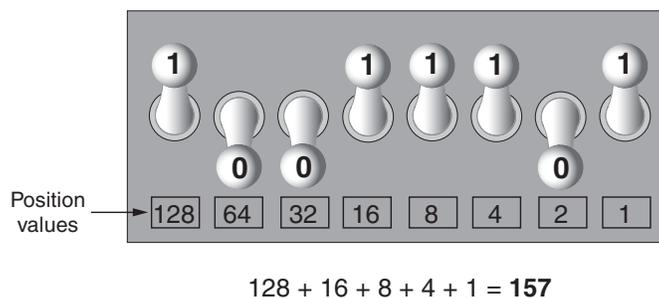
When all of the bits in a byte are set to 0 (turned off), then the value of the byte is 0. When all of the bits in a byte are set to 1 (turned on), then the byte holds the largest value that can be stored in it. The largest value that can be stored in a byte is  $1 + 2 + 4 + 8 + 16 + 32 + 64 + 128 = 255$ . This limit exists because there are only eight bits in a byte.
