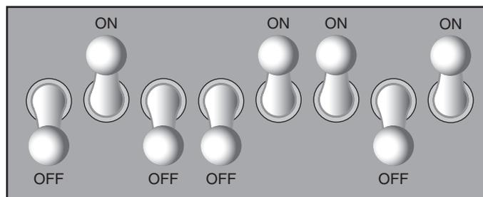
When a piece of data is stored in a byte, the computer sets the eight bits to an on/off pattern that represents the data. For example, the pattern shown on the left in Figure 1-8 shows how the number 77 would be stored in a byte, and the pattern on the right shows how the letter A would be stored in a byte. We explain below how these patterns are determined.
