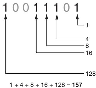
Figure 1-12 shows how you can picture the number 157 stored in a byte of memory. Each 1 is represented by a bit in the on position, and each 0 is represented by a bit in the off position.
