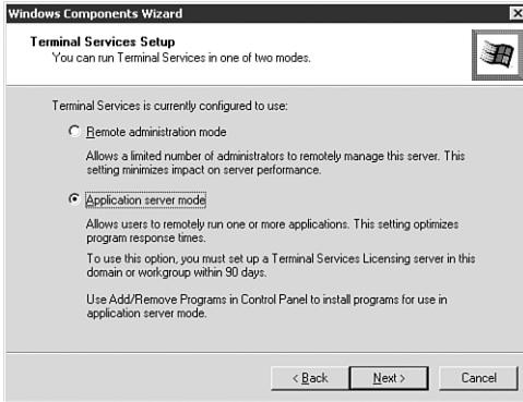
Figure 3.2 Terminal Server Mode selection screen.
