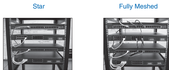
Figure 1-19 Star and Full-Meshed Topologies
